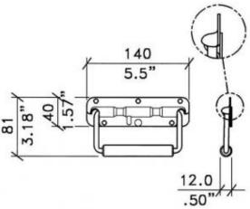
FIXING HOLES 5mm / .20" DIA
